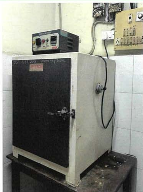
Plate 18: Hot air oven of chemistry lab
