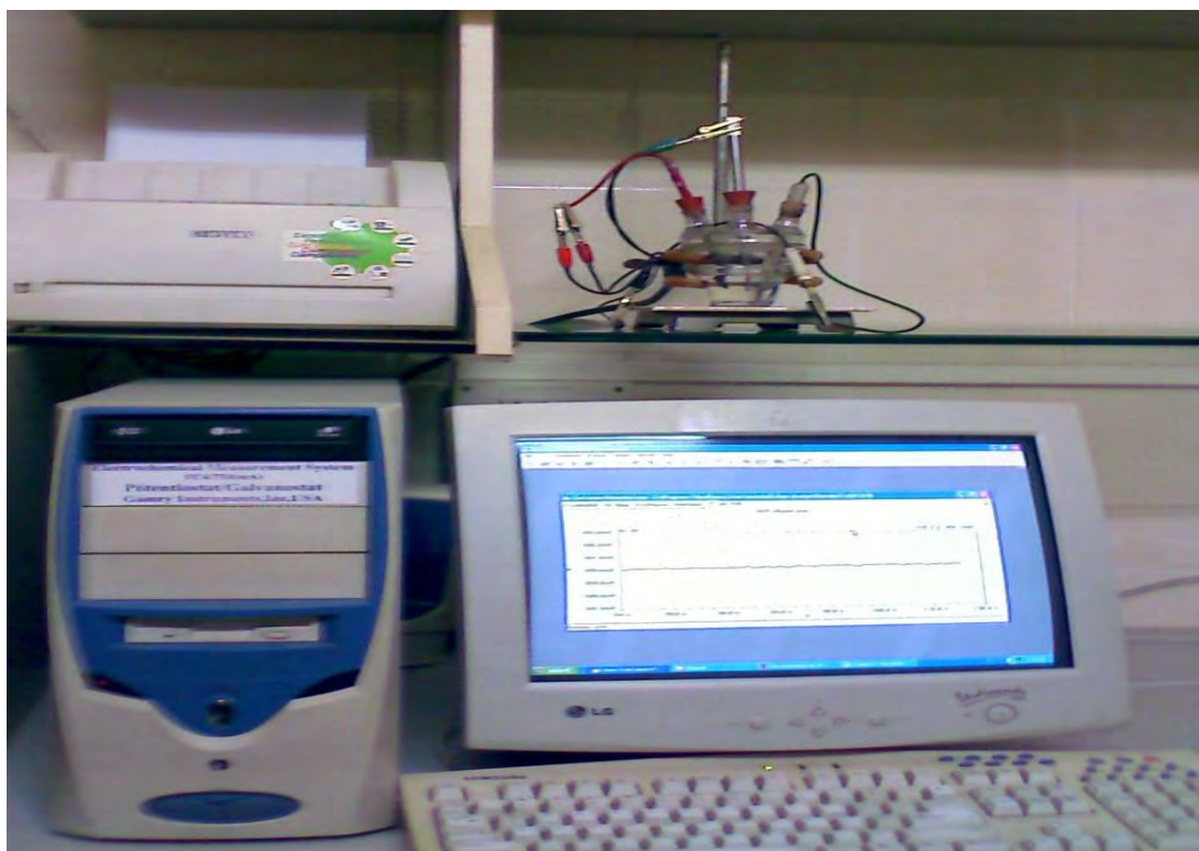
Figure 2.3: Electrochemical Measurement System, DC-105, DC corrosion techniques M/S Gamry instruments, Inc, USA.
