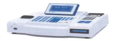
Biochemistry Analyzer is a medical laboratory equipment used extensively in clinical laboratories. It is designed to conduct tests to measure chemicals at various stages of the biological processes on a wide range of test samples from blood, plasma, serum, and cerebrospinal fluid to urine. In other words, it helps to study, analyze, and evaluate the characteristics of different body samples and tackle a broad of medical industry challenges.
